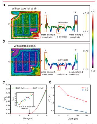
**Figure 4.** Piezo-phototronic effect modulated self-heating effect in LEDs. Infrared thermography showing the temperature rise  $\Delta T_j$  of different areas at 7 V bias voltage (a) without external strain and (b) with external strain. (c) I-V curve under different strain control, and the current under different strains at 4 V bias voltage. (d) The relationship between temperature rise  $\Delta T_j$  and external strains at 6 and 7 V bias voltages.
