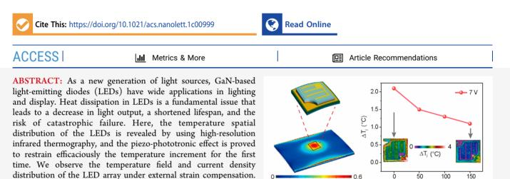
Depth (µm) external strain (GPa) Specifically, the temperature rise caused by the self-heating effect is reduced by 47.62% under 0.1% external strain, which is attributed to the enhanced competitiveness of radiative recombination against nonradiative recombination due to the piezo-phototronic effect. This work not only deepens the understanding of the piezo-phototronic effect in LEDs but also provides a novel, easy-to-implement, and economical method to effectively enhance thermal management.
