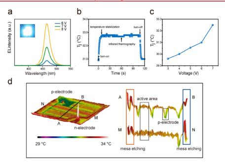
**Figure 3.** Self-heating effect of LED devices. (a) EL spectra of LED measured under different applied voltage. (b) The junction temperature  $(T_j)$  as a function of time and (c) applied voltage. (d) Infrared thermography showing the junction temperature  $(T_j)$  of different areas at 7 V bias voltage as well as a partial enlarged view.
