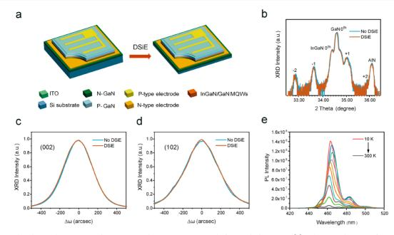
**Figure 1.** Optical and crystal properties of  $In_{0.16}Ga_{0.84}N/GaN$  MQWs LEDs before and after DSiE. (a) Schematic diagram of LED device before and after DSiE. High-resolution XRD: (b)  $2\theta$ - $\omega$  scans, (c) symmetric (002), and (d) asymmetric (102)  $\omega$ -scan rocking curves. (e) PL spectra under various temperatures from 10 to 300 K.
